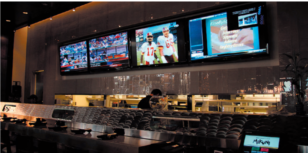
For customers entering Mikuni Restaurant, the first view is of four 65" LCD displays creating a massive videowall driven by the WindoWall System and a MAV Plus 1616 HD matrix switcher.
