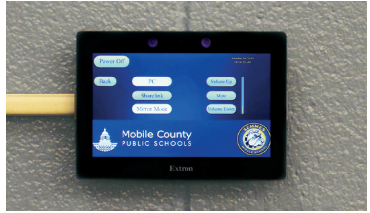
The TouchLink control system handles power on/off, which content to show, and audio volume.
