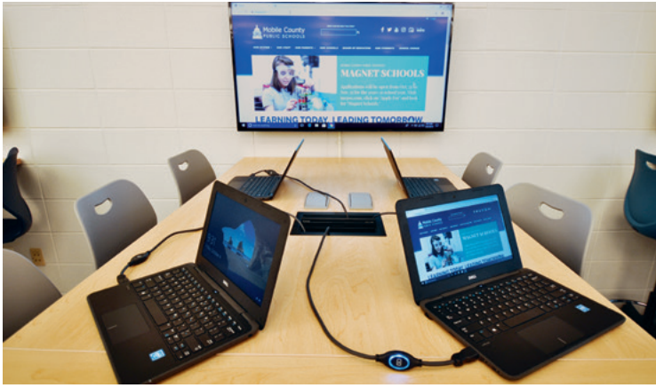
Students display their content by simply pushing the Share button on their TeamWork Show Me cable.
