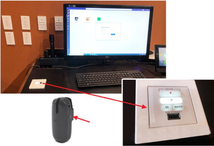
RCP 101 Remote Control Panel for SMP 351 Streaming Media Processor is located on the AV operator desk, providing a convenient location to insert a USB memory stick and to start, stop, pause, lecture capture and streaming. Presenters can also control start, stop, and pause from a button on their VoiceLift Pro pendant mic.
