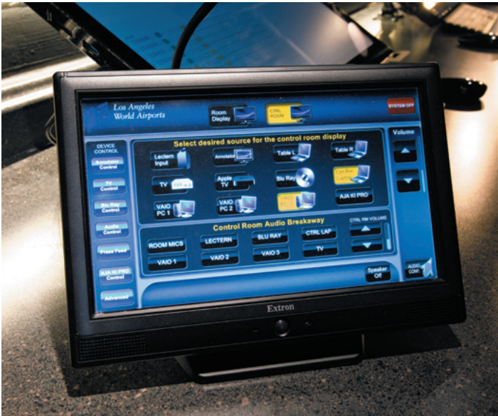
TouchLink touchpanels enable AV system operation and monitoring from the lectern and the control room.
