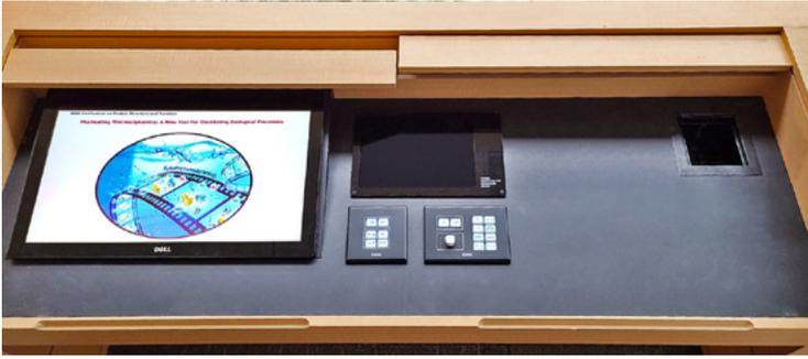
The lectern. Button panels plus an interactive touchpanel GUI on an iPad comprise the VTC-AV user interface. The lectern PC's display is at left. A guest laptop can connect via an Ethernet cable in the compartment upper right. Photo courtesy of Neuroo Digitech.
