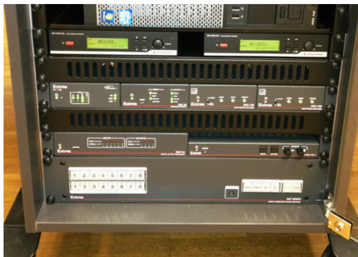
The Extron DXP 84 HDMI Matrix Switcher and other equipment conveniently mounted in the lectern.
