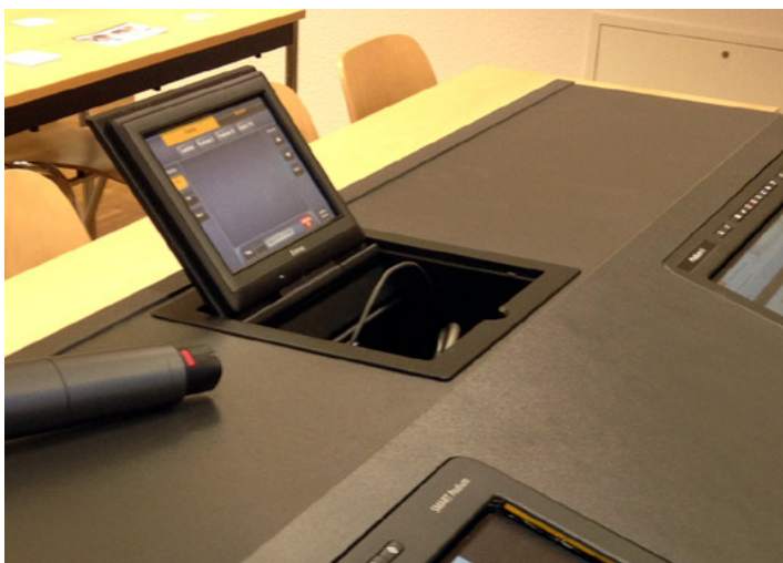
The TLP 710CV TouchLink Touchpanel flips up to provide complete access to system controls at the lectern.
