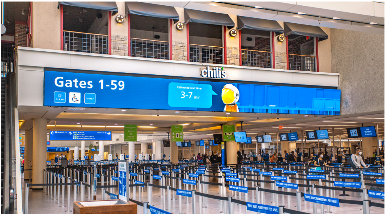
Media servers are located throughout the airport and the high resolution HDMI signals are extended to all of the displays over twisted pair cabling using Extron DTP transmitters and receivers. To watch a background video clip about the virtual aquarium that Synect created for the GOAA, click here .
