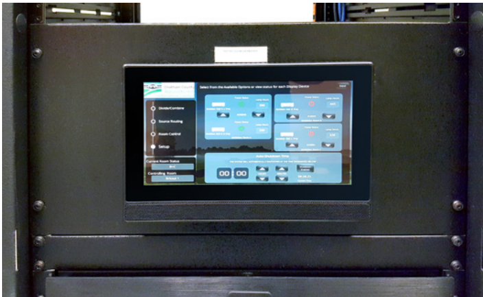
This Extron TLP Pro 1022M 10" Wall Mount TouchLink Pro Touchpanel displays the custom interface designed to control I/O source devices available on CCACC's XTP system.
