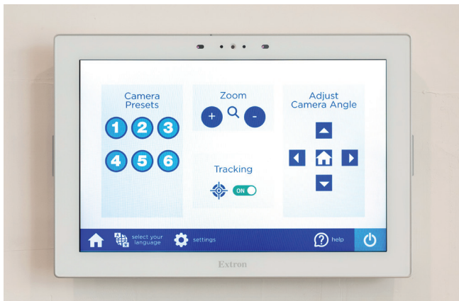
KONTEK used GUI Designer software from Extron to create the custom user interface, which is intuitive for users of all experience levels.
