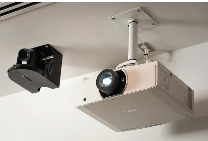
The compact NAV scaling decoder is installed close to the ceiling mounted projector.
