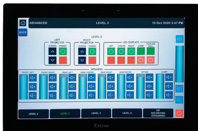
Touchscreen graphical interfaces allow operators to easily configure the mosque's AV system to accommodate prayer services, classes and special events (Photo courtesy of Hazelbayu Studios Pte Ltd).
