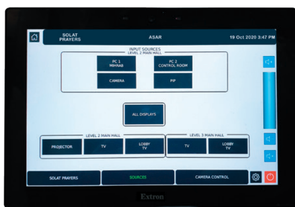
Touchscreen graphical interfaces allow operators to easily configure the mosque's AV system to accommodate prayer services, classes and special events (Photo courtesy of Hazelbayu Studios Pte Ltd).
