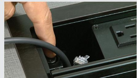
HOLD CONNECTOR AND PUSH RELEASE BUTTON, TO STORE CABLE BACK IN THE ENCLOSURE
