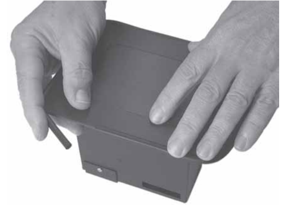
Figure B-2 — Installing protective strips
