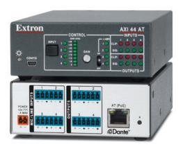
The Extron AXI 44 AT is a quarter rack width audio interface for integrating four mic/line sources onto a Dante<sup>™</sup>-enabled audio system. It features four mic or line inputs with switchable 48 volt phantom power. Input select, gain, and phantom power settings are controllable from the front panel, via DSP Configurator Software, or by SIS command.
